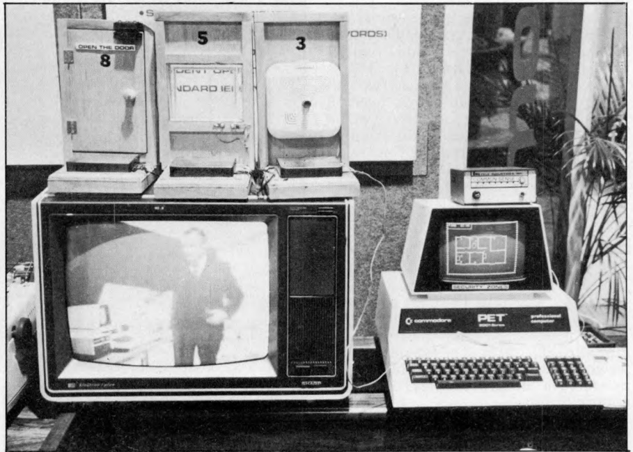
Left: Commodore's acoustic modem will let PETs converse over long distance telephone. Below: Common Sense security system — PET monitors alarm and displays security zones on screen.
